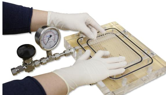
5. Place a piece of pre-cut membrane over the feed spacer using the four guideposts to hold the membrane in position. The membrane should be installed with the shiny or active side down toward the feed spacer.
