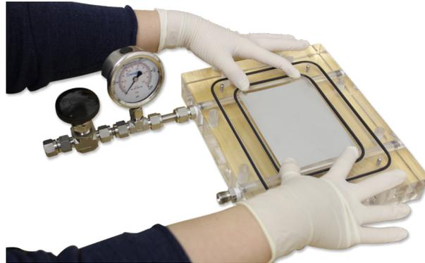
**Note:** Using Shims and Spacers enables to change the hydrodynamic conditions in the cell or to create a support for the membrane.
