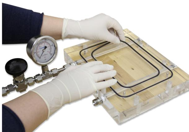
**Caution:** Make sure that the O-rings lie flat in the grooves of the cell bottom. Leaking may occur if the O-rings do not lie flat in the grooves. The O-rings will be cut or crushed when the system is operating if the O-rings are not installed correctly.
