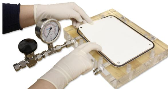
**Note:** If you are cutting your own membranes, the membrane's outer edge should fit between the inner and outer O-rings in the cell body to prevent leakage.
