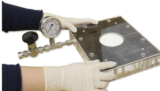
**Note:** The aperture in the acrylic spacer is designed for permeate outlet. It should be placed toward the permeate collection vessel.
