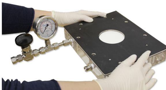
9. Place the Aluminum condenser plate over the gasket.
